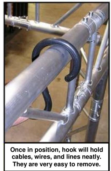
Once in position, hook will hold cables, wires, and lines neatly. They are very easy to remove.
